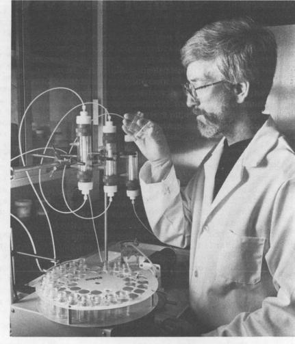
ION CATCHERS — Researchers at Sandia and Texas A&M, including Dan Trudell (6212), have engineered new crystalline silicotitanate materials that can extract radioactive cesium ions from the nonradioactive constituents of radioactive waste. Cesium has historically been one of the most difficult radioisotopes to remove from sodium-bearing waste such as that contained in underground tanks at the Hanford "tank farm," DOE's top environmental remediation priority. (Photo by Randy Montoya)
